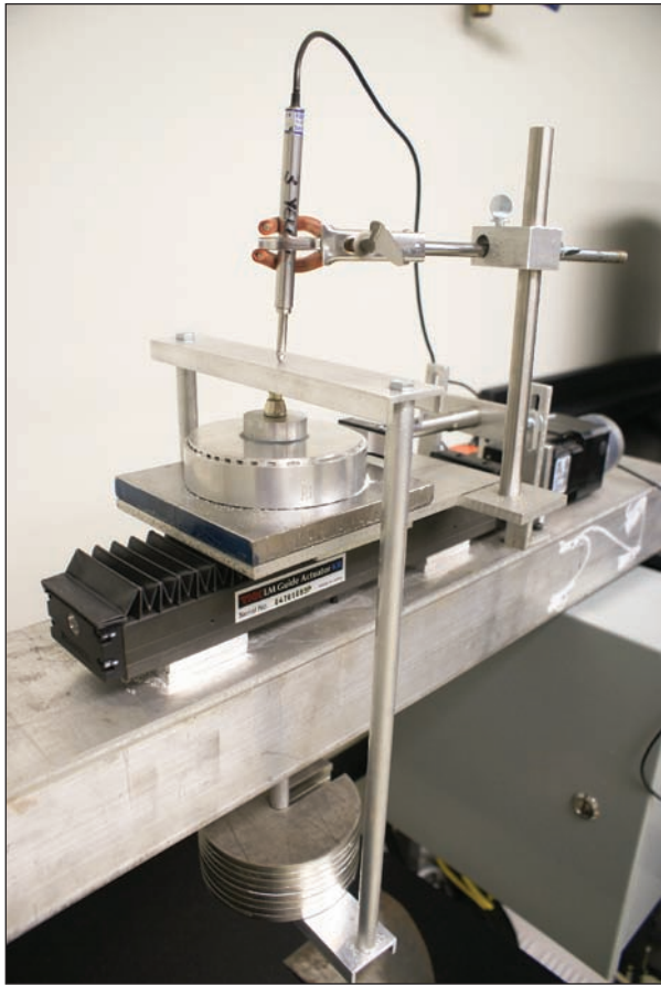
The direct shear tester will pull across a confined material under various applied pressures and moisture contents to determine the material's friction, cohesion, and adhesion to a substrate such as a liner material.
