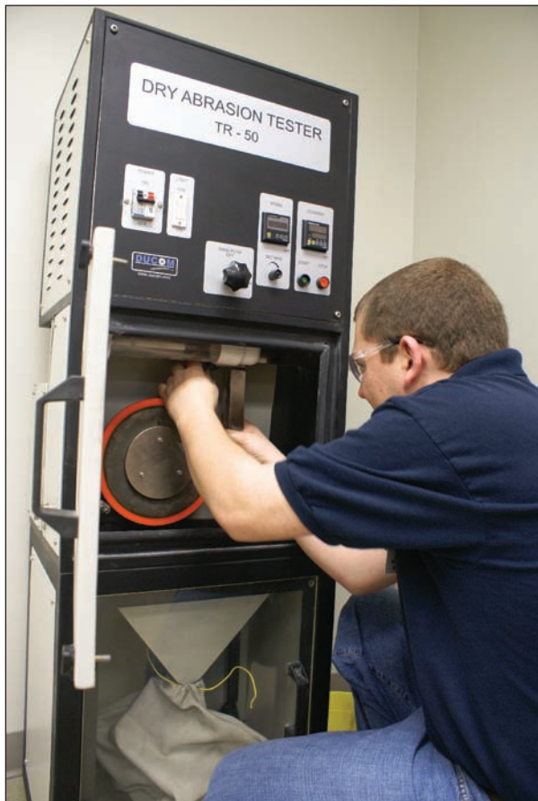
By running an abrasive (like sand) between a rubber disk and a sample of material, the dry abrasion tester checks three-body abrasive wear, as between a conveyor belt, a metal chute liner, and the bulk material.
